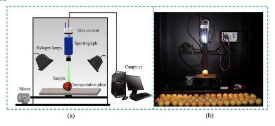
Figure 14 Schematic diagram and physical diagram developed by Dr. Zhang Baohua of Shanghai Jiaotong University; (a) Schematic diagram; (b) Physical diagram
