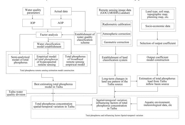
Figure 33 Inversion algorithm flow of hyperspectral data
