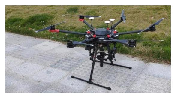
Figure 16 Drone-borne hyperspectral imaging camera
